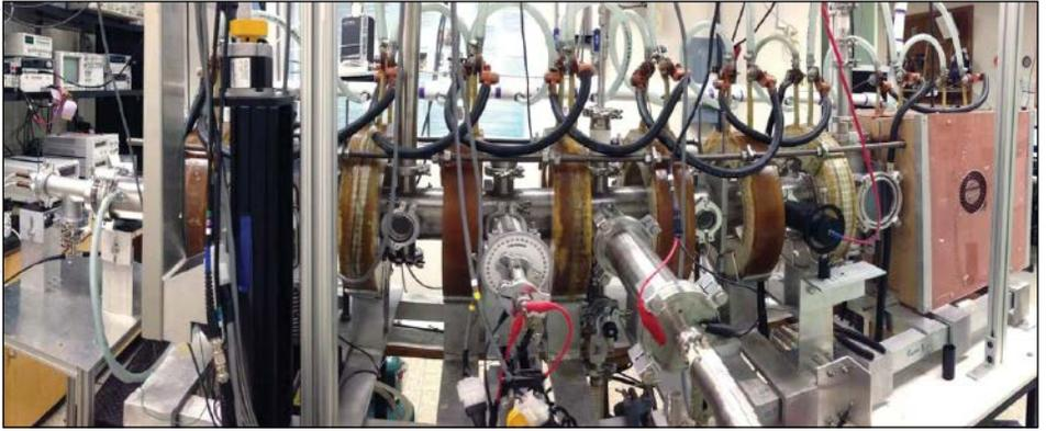
The Auburn Linear Experiment for Instability Studies (ALEXIS) helps scientists understand the factors that produce broadband electrostatic noise in boundary layers of the Earth's magnetosphere.
