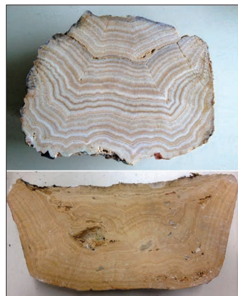
Two samples of sinter from Roman aqueducts, showing distinct banded layers. These layers typically represent seasonal cycles.
