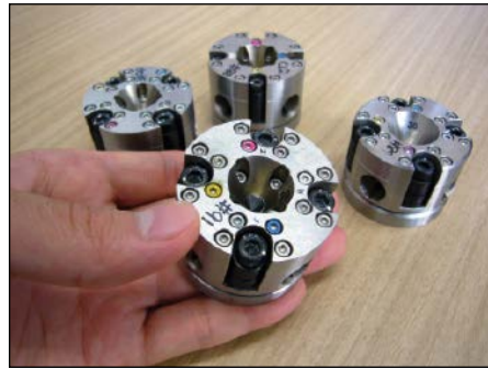
Diamond anvil cells (shown above) and laser heating were used to simulate the conditions of the lower mantle.
