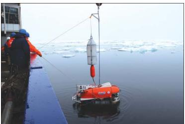
Nereid Under Ice vehicle being deployed from Polarstern during summer 2014.
