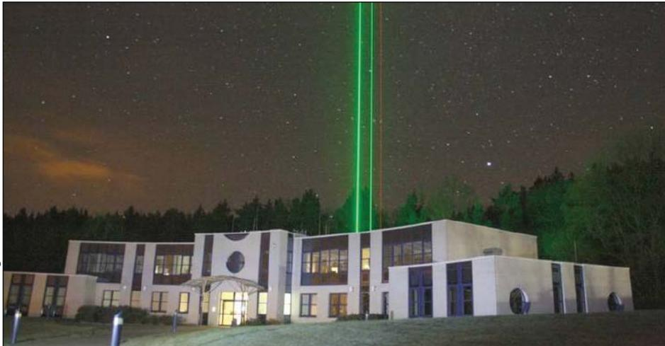
Laser beams of the ground-based lidar instruments at the Leibniz Institute of Atmospheric Physics in Kühlungsborn, Germany, slice through to an altitude of about 120 kilometers, collecting data in atmospheric regions along the way.
