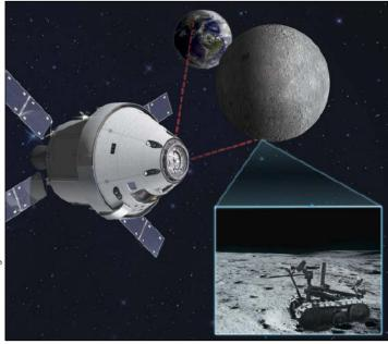
In a concept using NASA's new Orion crew vehicle, astronauts would orbit above the lunar farside and remotely operate a robotic vehicle while maintaining communication with Earth. Samples collected by a rover would be launched to Orion, where they would be stowed before the crew returned to Earth. in the Orion spacecraft. In this plan, Orion would hover above the Moon's farside around Earth–Moon Lagrange position L2.
