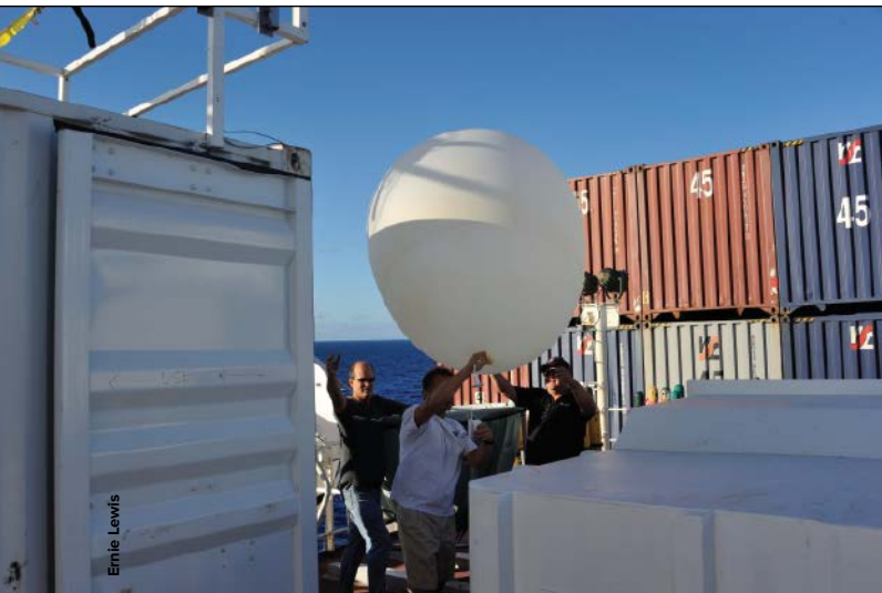
On the bridge deck of the Spirit cargo ship, members of the Marine ARM GPCI Investigation of Clouds (MAGIC) research team prepare to launch a balloon-borne radiosonde to take atmospheric measurements.
