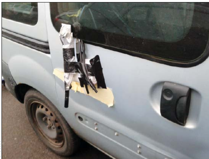
Air intake tubes dangle from a side window of an instrument-laden minivan that researchers used to chase vehicles on Slovenian roads while measuring their tailpipe emissions. The tubes fed exhaust gases into separate instruments for measuring black carbon, nitrogen oxide, carbon dioxide, and particulates.
