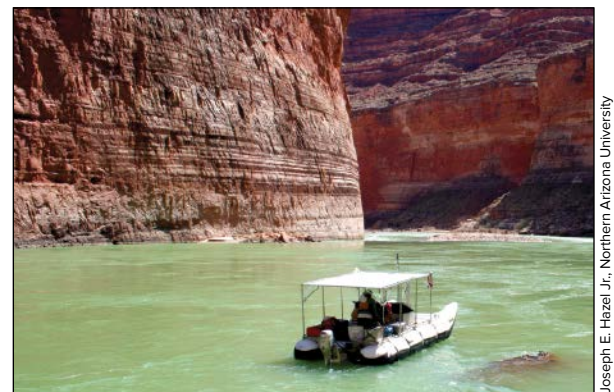
Scientists survey from a boat at a study site along the Colorado River within the Grand Canyon, collecting high-frequency acoustic backscatter data with a multibeam echosounder to determine riverbed grain size.
