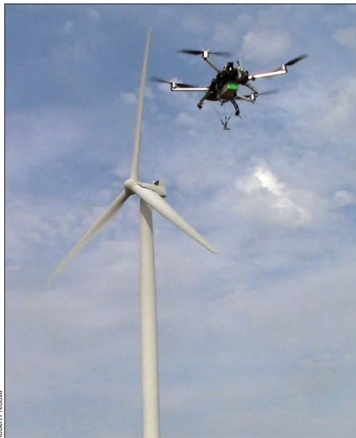
A remotely controlled quadcopter carries a temperature-sensing fiber-optic cable to investigate atmospheric mixing in an active wind farm.
