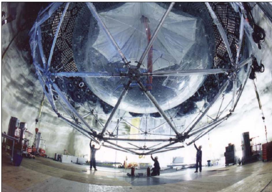
The detector at the heart of the Sudbury Neutrino Observatory, shown under construction in the mid-1990s, used a clear tank filled with heavy water surrounded by a shell of photodetectors to record neutrinos emitted by the Sun. The observatory's measurements showed that the Sun was generating as many neutrinos as predicted but that most of the particles were transforming from one kind of neutrino into another as they sped to Earth.
