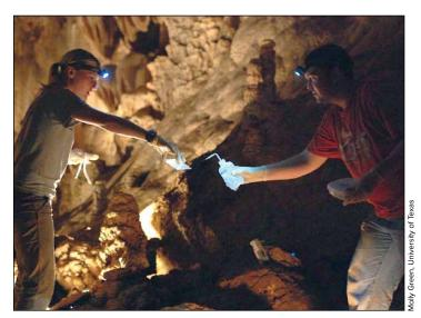
University of Texas researchers collect a glass substrate used to measure the amount of calcite deposited by cave drip water in Natural Bridge Caverns, Texas.
