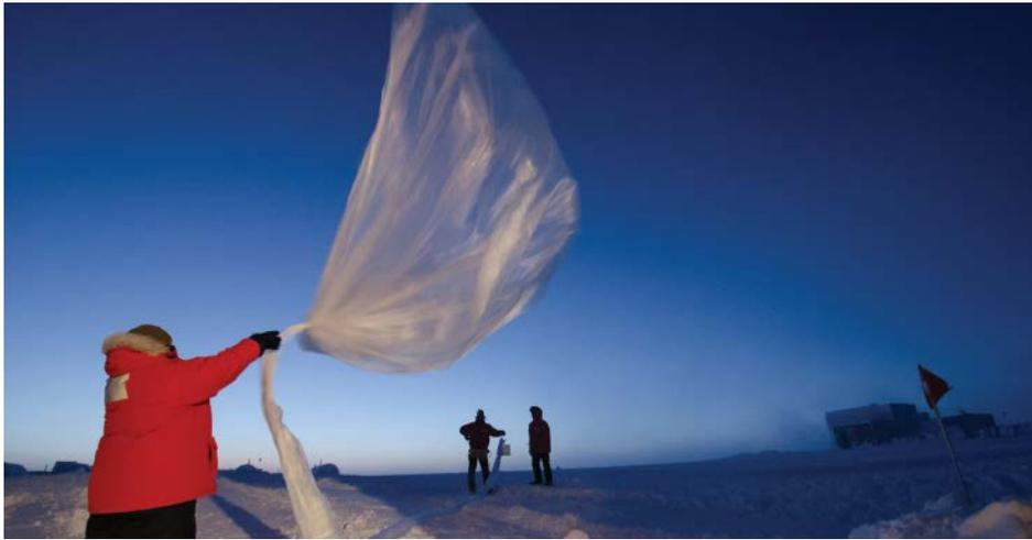
Researchers launch an ozonesonde in 2013. These balloon-borne instruments provide information on ozone and meteorological quantities such as pressure, temperature, and humidity.
