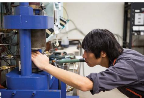
A visiting postdoc prepares for a high-pressure experiment in Texas A&M's John W. Handin Laboratory for Experimental Rock Deformation. The instrument pictured here is a triaxial Griggs deformation apparatus, which allows scientists to perform compression experiments at pressures and temperatures of the middle crust to upper mantle.
