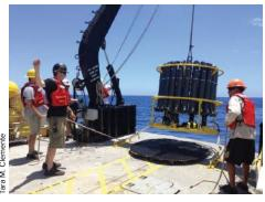
Deploying conductivity-temperature-depth instruments from R/V Oceanus for Hawaii Ocean Time-Series cruise 284 in May 2016.
