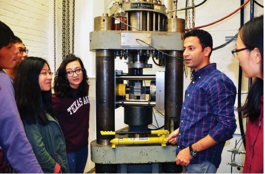
Graduate and undergraduate students gather in a Texas A&M laboratory to learn how friction experiments are done at sliding velocities of up to 1 meter per second. Energy dissipation at these velocities initiates dynamic weakening processes that govern earthquake rupture.
