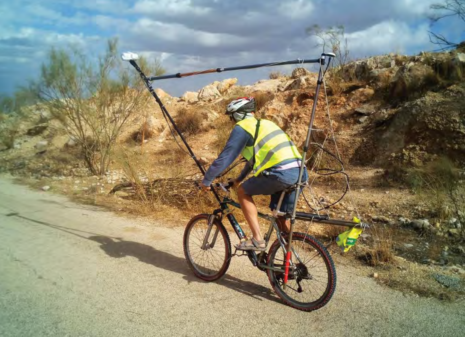
Uri Schattner tests the bike-mag system across the shoulder of the Dead Sea fault valley in northeastern Israel. Credit: Amit Segev
