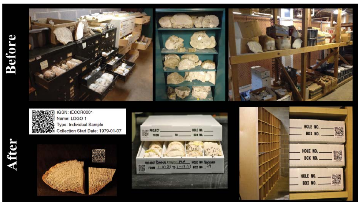
Fig. 1. Lamont-Doherty Core Repository at Columbia University before and after organizing coral samples in boxes. Each sample was given an IGSN and Quick Response (QR) code for the storage box so that core pictures, X-ray images, and other available information can be linked to the samples. Credit: Emilie P. Dassié and Michael Sandstrom
