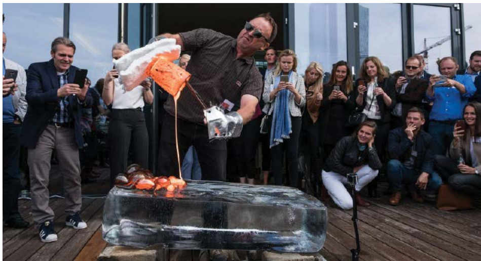
Artist Bob Wysocki pours homemade basaltic lava over ice at a demonstration in Reykjavik, Iceland. Steam released from the ice by the sudden heating inflates bubbles in the lava that solidify into glass shells as the lava cools. Credit: Syracuse University Lava Project
