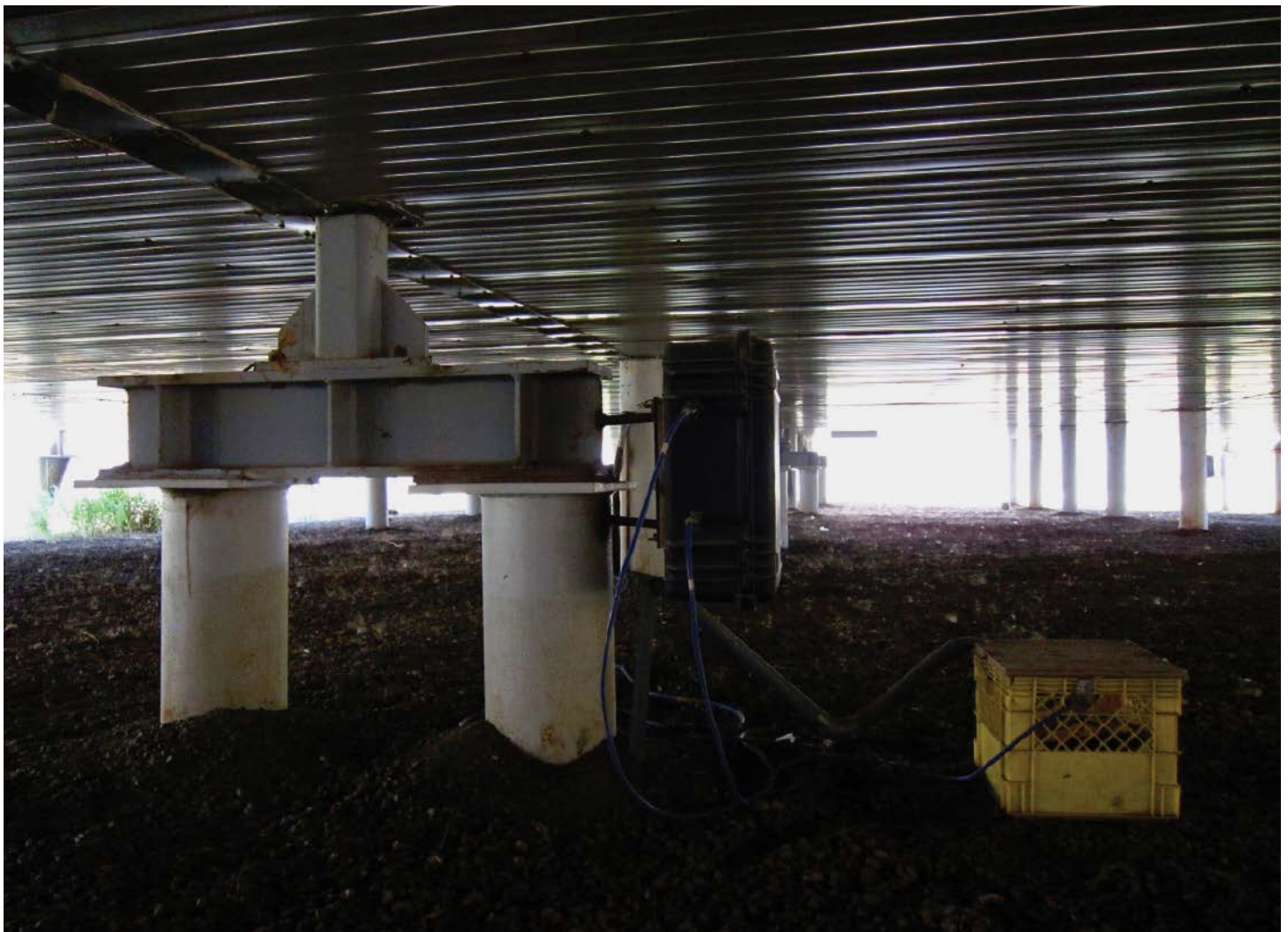
Beneath the Aurora Research Institute's two-story building in Inuvik, researchers have installed a series of experimental pilings and ground temperature monitors to test best practices in preserving the permafrost below and maintaining the structural stability of the building. Credit: Laura Poppick
