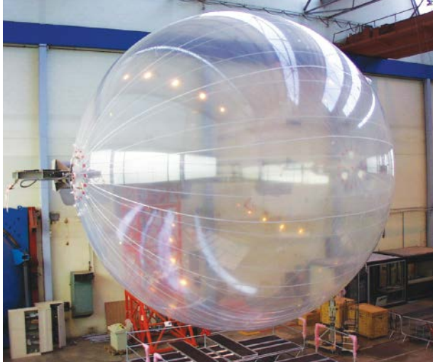
A fully inflated superpressure balloon in the lab at the French National Center for Space Studies. Credit: Philippe Cocquerez, CNES
