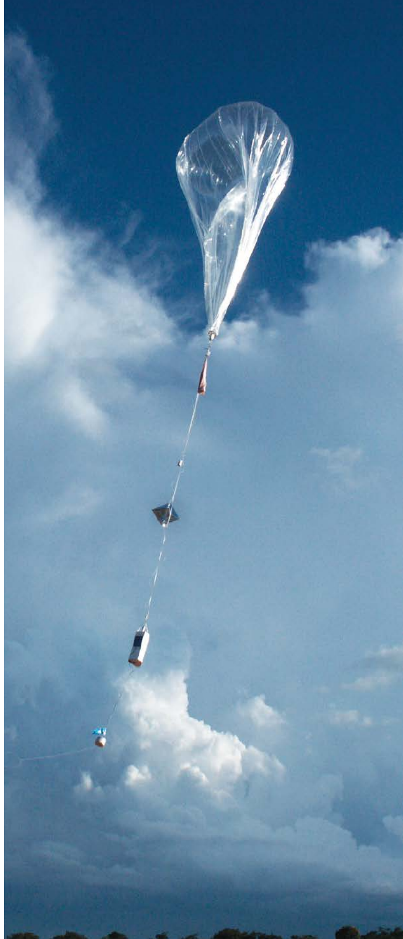
This superpressure balloon, shown here at launch, is not fully inflated. As it rises, the volume of helium sealed inside increases until the spherical balloon is fully inflated, giving it a fixed density. Once the balloon has reached the atmospheric level where the air has the same density, it drifts with the wind, providing accurate wind measurements.
