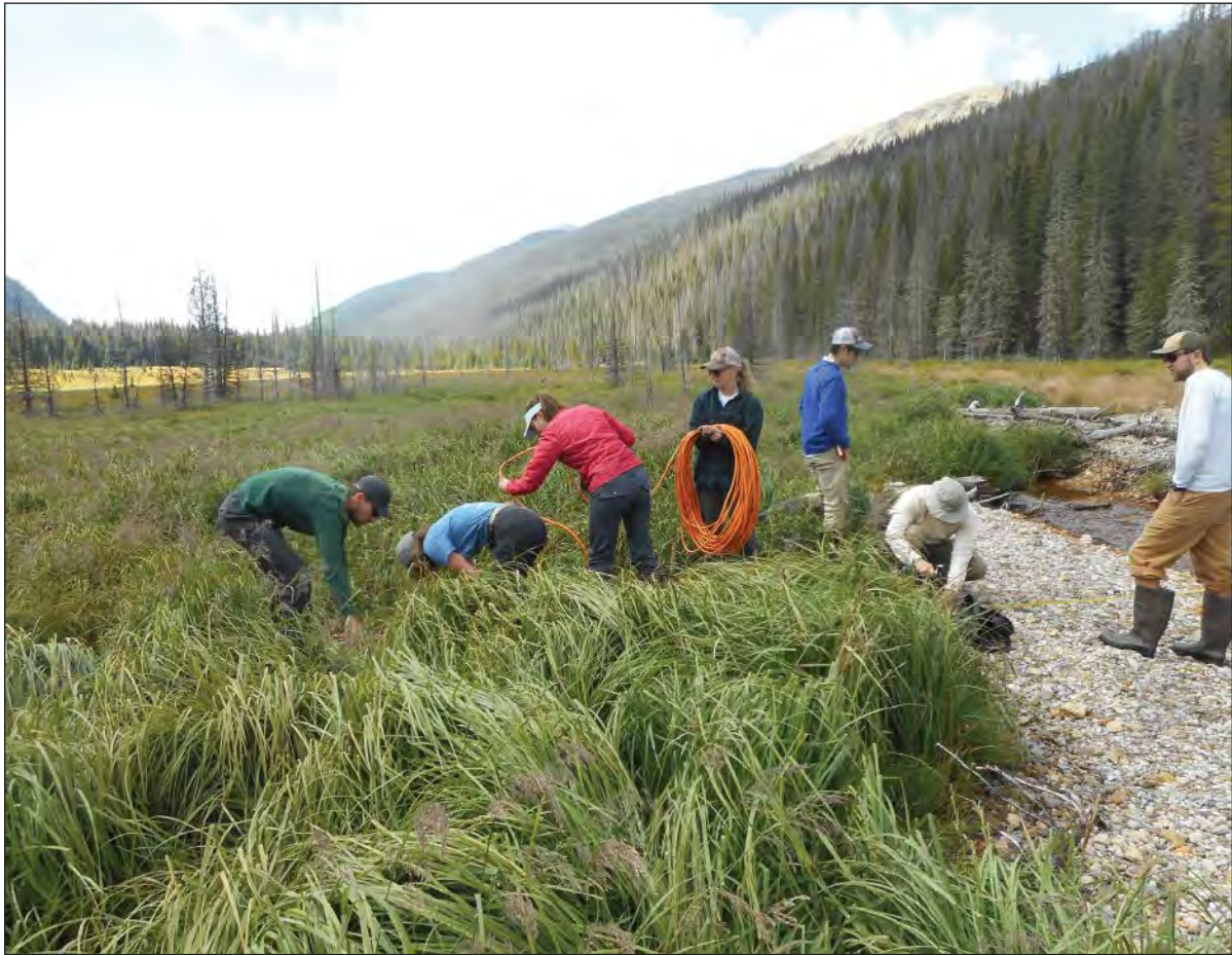
Students lay cables for an electrical resistivity survey within a wetland along the Colorado River in Rocky Mountain National Park. Credit: Sara Rathburn
