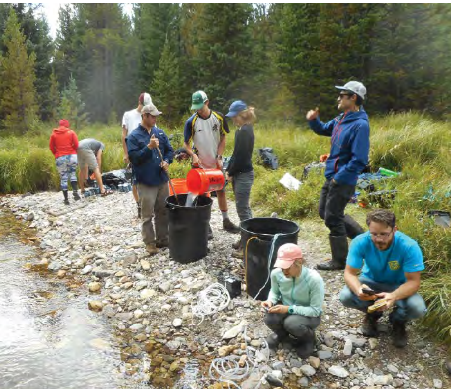
Graduate and undergraduate student volunteers from Colorado State University test the pumping rate during a conductivity tracer test at a local research hub on the upper Colorado River in Rocky Mountain National Park. Credit: Sara Rathburn
