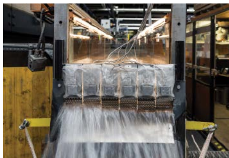
As water runs out of a flume, particles of sediment strike impact plates. Researchers record these vibrations to measure sediment transport. Credit: Bob de Graffenried
