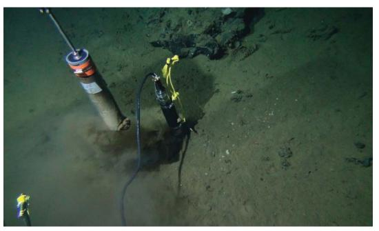
A photograph taken from Alvin, a manned deep-ocean research submersible, of sediment coring on the ocean floor at Dorado Outcrop in 2014. Credit: NSF OCE 1130146 and the National Deep Submergence Facility
