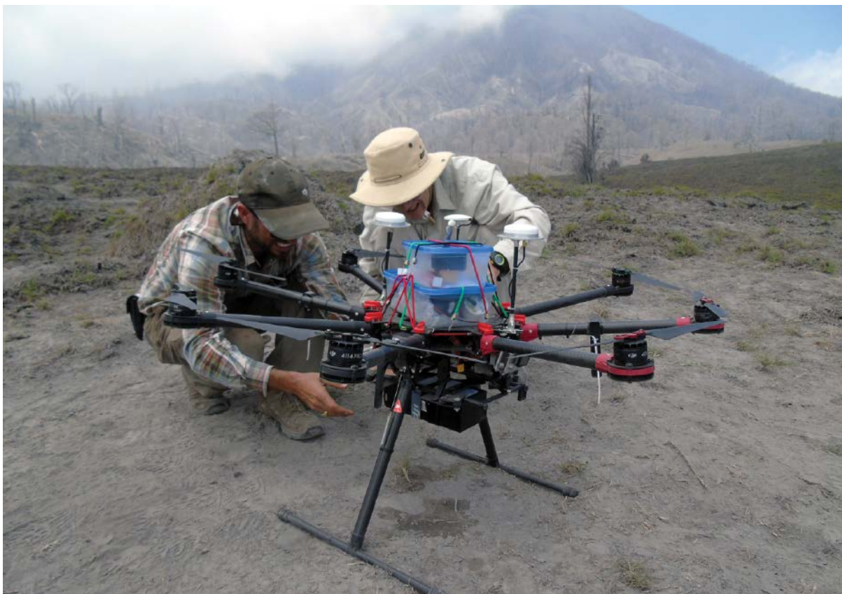
Researchers make final adjustments to a drone equipped with compact gas instrumentation. The drone will carry the instruments through the gas plume emitted by Turrialba volcano, seen here behind the researchers. Credit: Fiona D'Arcy
