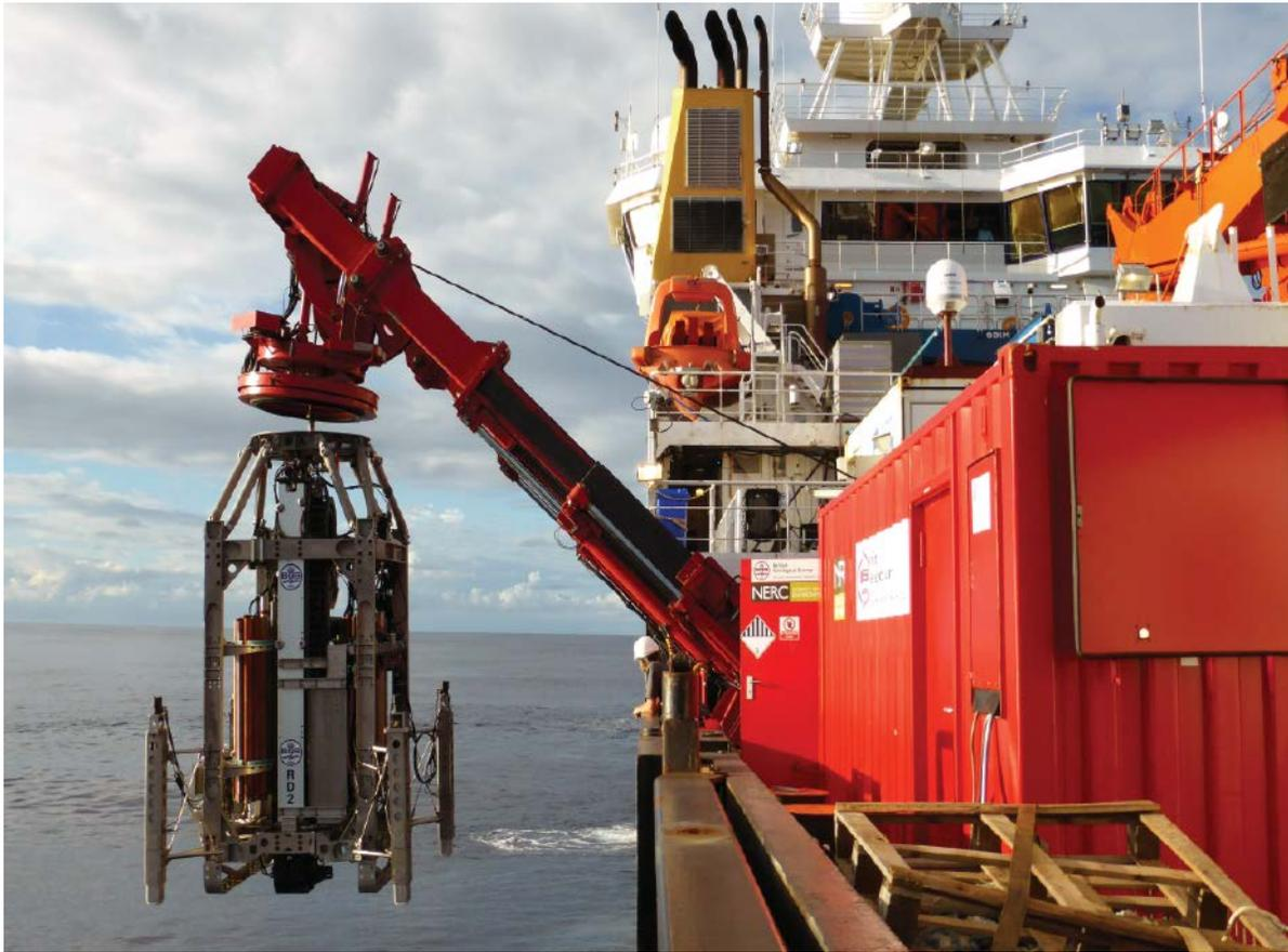
ODP Expedition 357 used seabed drills for the first time in the ocean drilling program. Here the RD2 seabed drill is deployed over the starboard side of the RRS James Cook. Credit: Dave Smith
