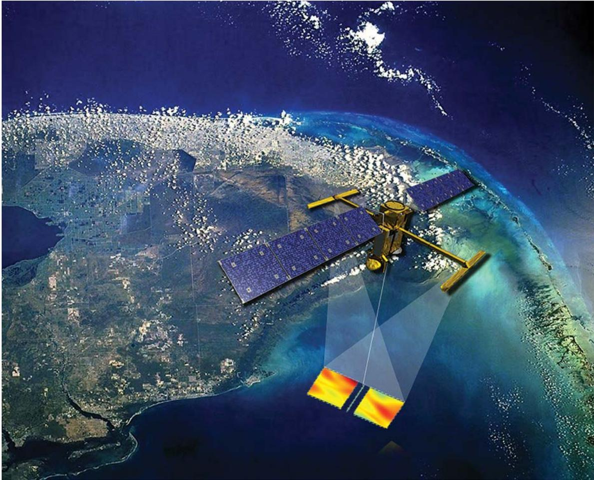
Artist's rendering of the future SWOT satellite making sea surface height observations, even through clouds. Off-nadir radar interferometers gather data over two 60-kilometer-wide swaths at once, with a conventional nadir altimeter in between. Credit: CNES
