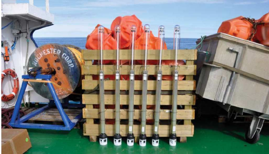
RAFOS floats aboard the R/V Hakon Mosby await deployment. These floats spend up to 2 years in the ocean, after which they surface and transmit their data to satellites. Scientists can then download the data directly to their computers. Credit: Marieke Femke de Jong
