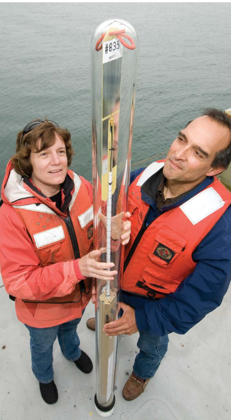
Amy Bower and a technician with a RAFOs float. Credit: Tom Kleindinst, © Woods Hole Oceanographic Institution
