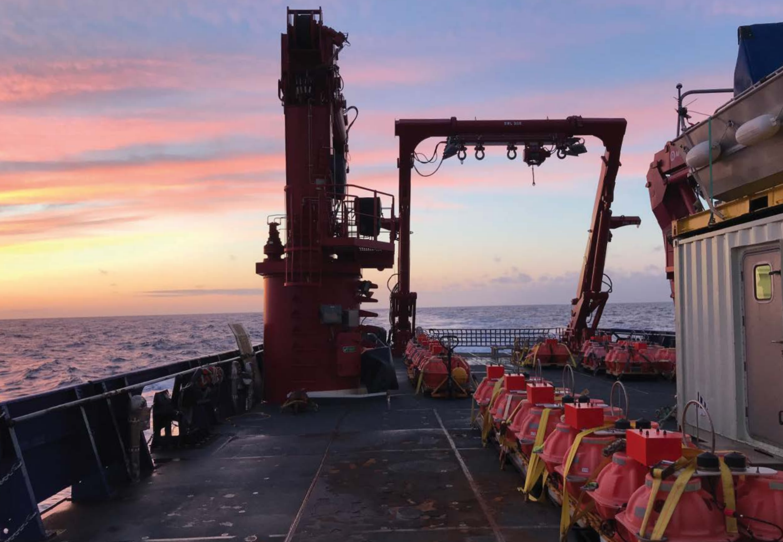
Sunset from the R/V Sikuliaq, July 2018. Broadband ocean bottom seismometers arranged on deck are ready to be deployed in support of the Alaska Amphibious Community Seismic Experiment. Credit: Anne Sheehan
