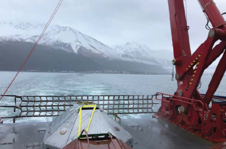
Fig. 2. Ocean bottom seismometers used in AACSE. A shallow-water instrument (left). Dan Kot prepares a deepwater OBS for deployment (right). Credits: David Heath (left); Anne Sheehan (right)
