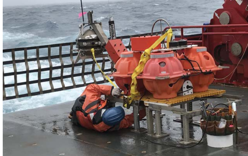
Fig. 2. Ocean bottom seismometers used in AACSE. A shallow-water instrument (left). Dan Kot prepares a deepwater OBS for deployment (right). Credits: David Heath (left); Anne Sheehan (right)
