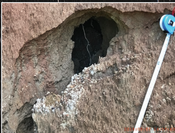
(left) Debris from a landslide as seen on 20 August 2018 butts against homes in Idukki, stacking dirt and vegetation onto roofs. Credit: I&PRD, Government of Kerala. (right) Researchers found this large hole in a landslide photographed on 7 September 2018 and believe it is evidence of a subsurface piping, which can destabilize hillslopes. Credit: Thomas Oommen
