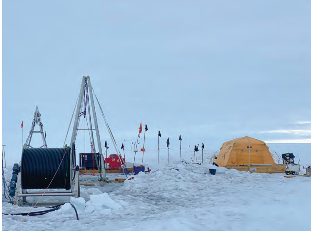
Researchers with the MELT project set up equipment, including an A-frame structure and a winch, to deploy instruments through a borehole in Thwaites at their research site in January 2020. Credit: David Holland
