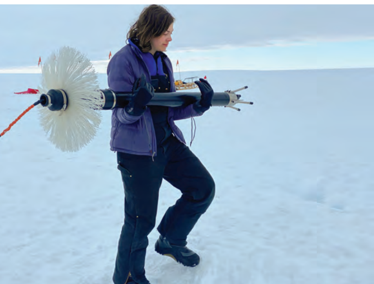
Aurora Basinski, a graduate student at New York University, carries a device for deployment through a borehole in Thwaites Glacier in January 2020 as part of the Melting at Thwaites Grounding Zone and Its Control on Sea Level (MELT) project. The instrument will measure water turbulence in the ocean beneath the glacier near its grounding zone. Credit: David Holland
