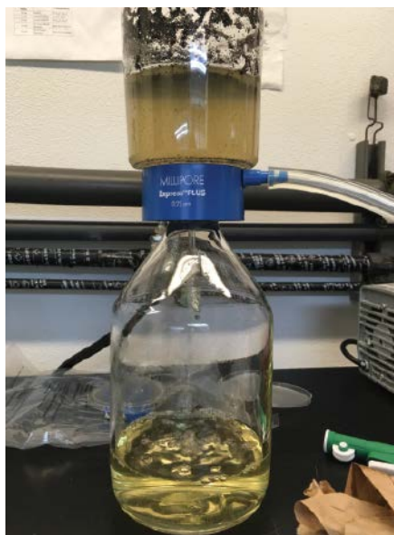
Researchers siphoned out the ash from the seawater after letting it soak for 1 hour. Credit: Tanika Ladd
