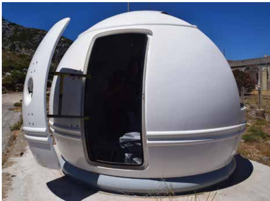
This 3-meter astronomical dome with Sun-tracking capabilities hosts the solar polarimeter (SolPol) instrument of the Panhellenic Geophysical Observatory of Antikythera (PANGEA). Credit: Stav Dimitropoulos
