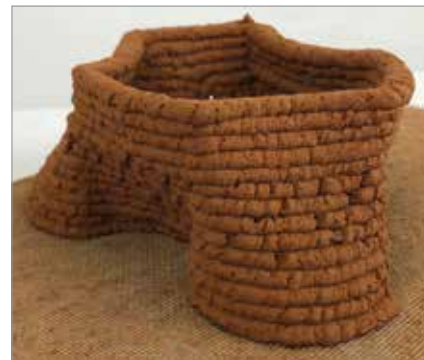
Scientists and engineers are developing soil-based concrete replacements like this prototype structure. Credit: Aayushi Bajpayee
