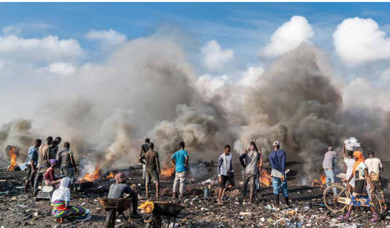
People burn wires, cables, circuit boards, and other discarded items to recover copper at the Agbogbloshie electronic waste site in Ghana. Credit: Muntaka Chasant, CC BY-SA 4.0 ( bit.ly/ccbysa4-0 )
