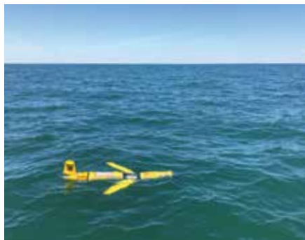
A Slocum glider operated by Rutgers University is deployed off the coast of New Jersey. Underwater gliders equipped with sensors provide live data that help scientists understand in real time how acidity is changing in Earth's oceans. Credit: Liza Wright-Fairbanks, Rutgers University
