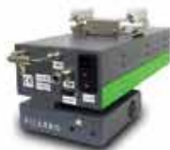
Micro-Combustion Module for plant and soil waters
