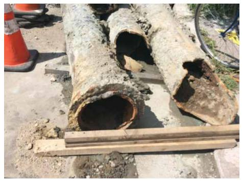
Natural gas can leak from crumbling cast-iron pipes under the city's streets. Cast-iron and steel pipes and joints are more than 50 years old in some places in Boston, and their sealants are cracking. Credit: Audrey Schulman
