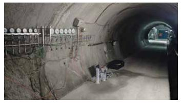
This photo from a tunnel at the Grimsel Test Site in Switzerland was taken during a geochemical sampling campaign to analyze changes in groundwater following microseismic events. Credit: Richard Lord
