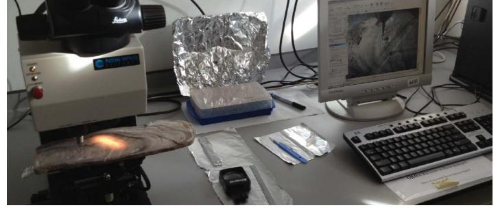
Samples are milled from a speleothem using a small drill. Credit: Nikita Kaushal
