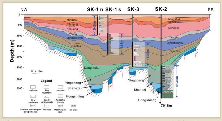
Fig. 2. Cross section of the Songliao Basin from northwest to southeast, showing named layers of sedimentary rock in the basin as well as the drilling and coring strategy of the three phases of the SK project.
