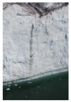
An image taken from a helicopter shows the deepwater sensor cable at the calving front being dragged away from the ice cliff by a strong underwater current created by a subglacial plume. Credit: Shin Sugiyama
