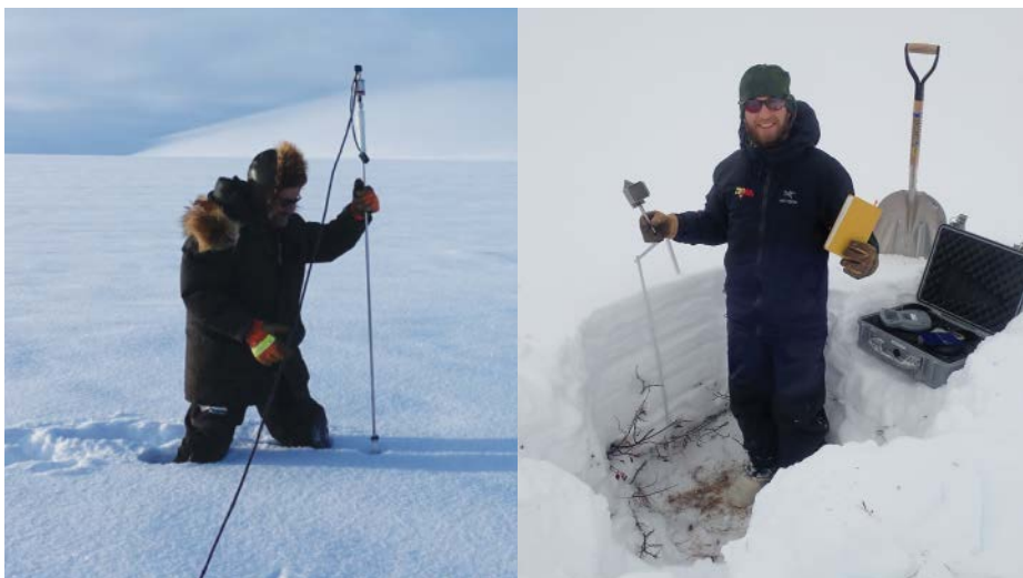
(left) Matthew Sturm, who specializes in tundra research, probes for snow depth using a GPS-enabled automatic depth probe. (right) Charlie Parr, a research technician at the University of Alaska Fairbanks, measures the density of layers of snow. Credit: Matthew Sturm
