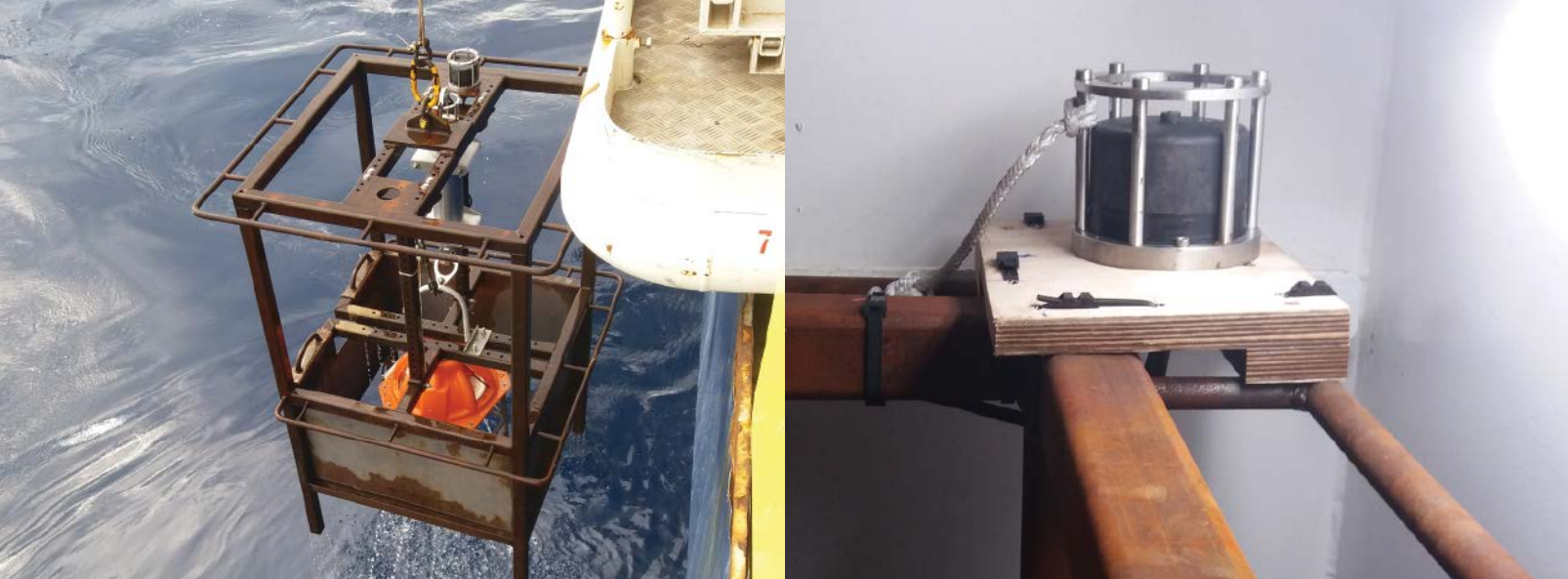
The ballast cage (left) is deployed over the side of R/V Pourquoi Pas?. The cylinder mounted to the top center strut is the acoustic transmitter of the Ultra Short Baseline (USBL) positioning system. For the last three OBS deployments, the acoustic transmitter of the USBL positioning system (right) was decoupled from the metal cage using a wooden plate and was moved from the top center to a corner of the cage for better communication with the ship. Credit: Pascal Pelleau
