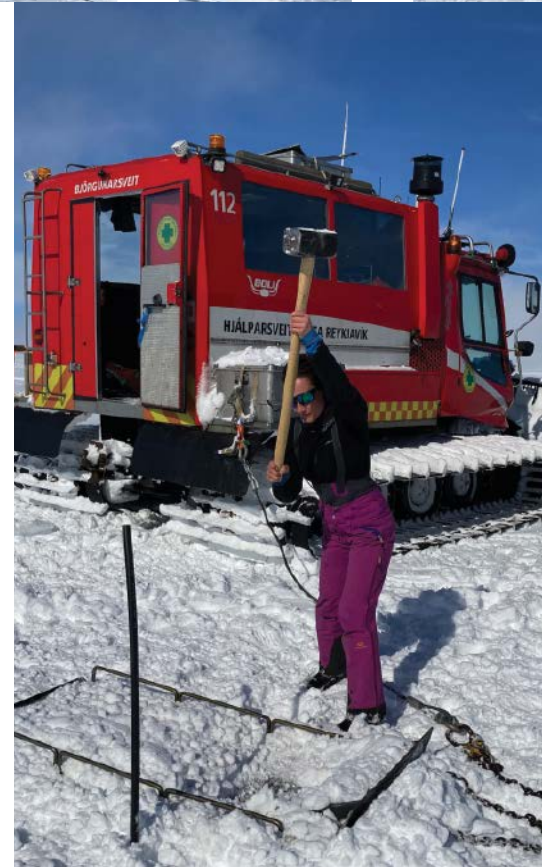
Sara Klaasen conducts a hammer test to create a seismic signal that the distributed acoustic sensing cable can record. To increase the strength of their hammer blows, the researchers pounded on the metal plate on the plow used to deploy the cable. Credit: Sölvi Thrastarson
