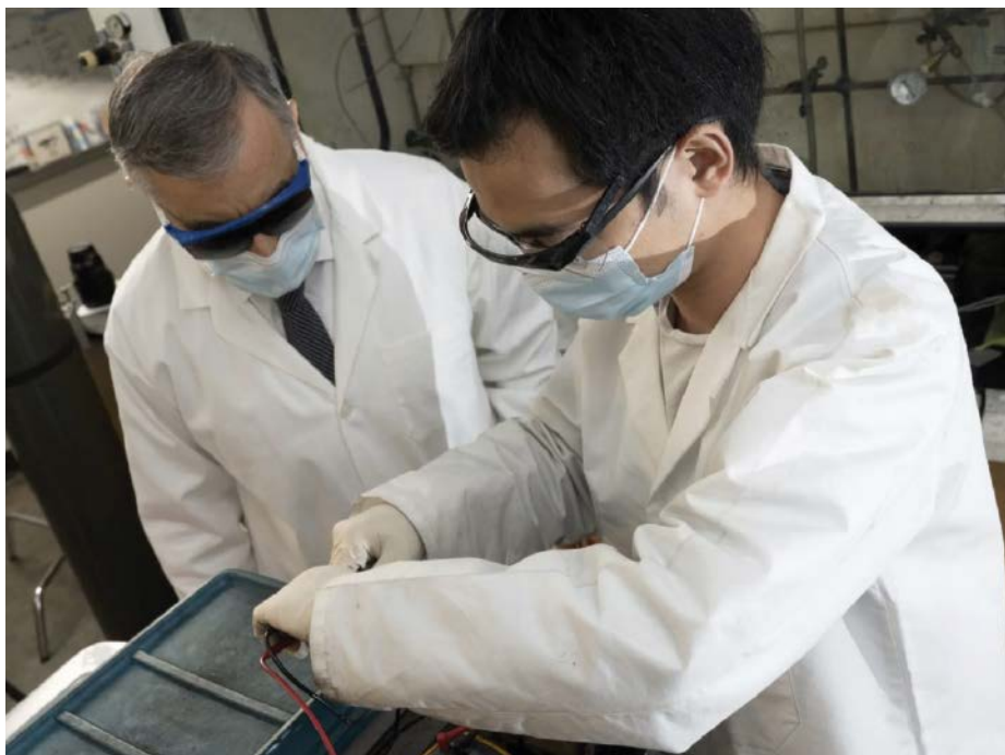
Rice University chemist James Tour (left) and postdoctoral researcher Bing Deng administer a jolt of electricity to some coal fly ash. The method could be used to turn this powdery waste material into rare earth elements needed for electronic devices. Credit: Jeff Fitlow/Rice University
