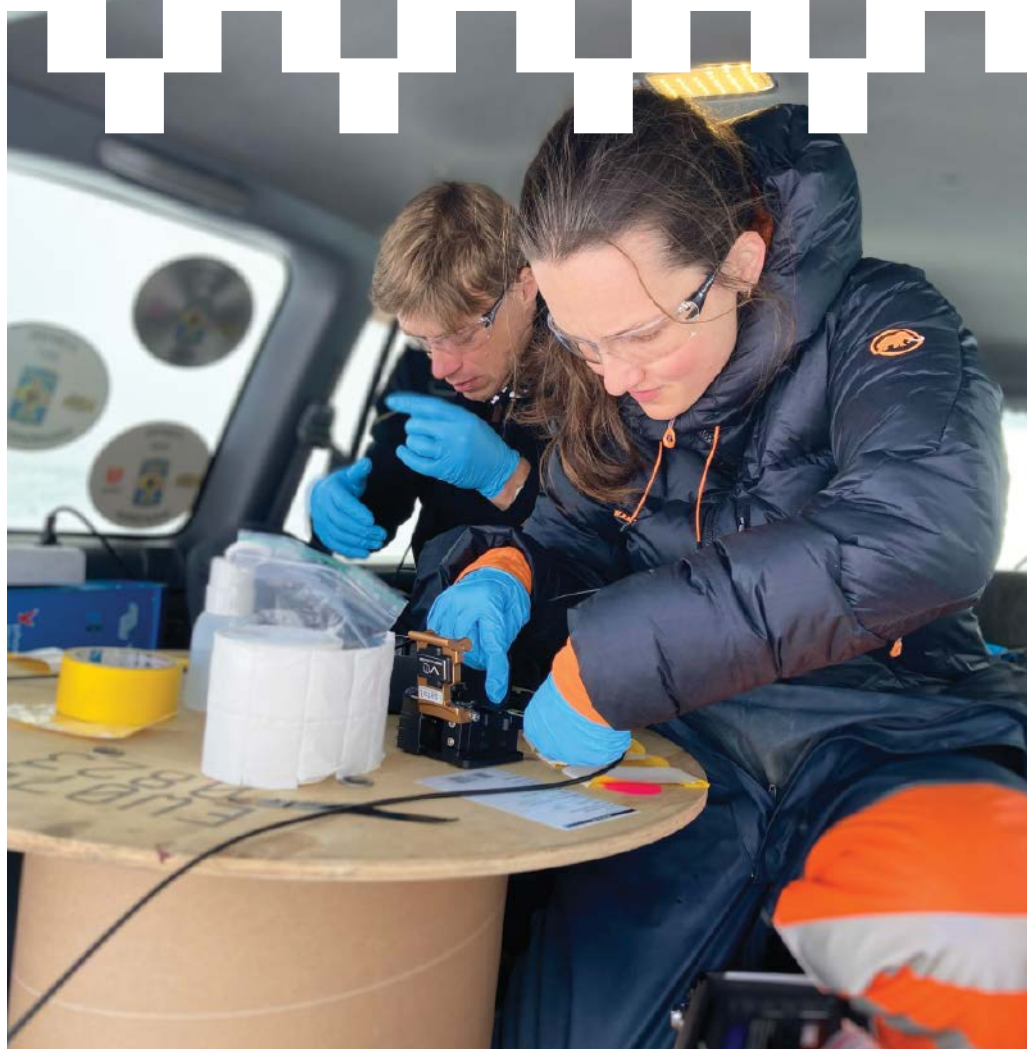
Andreas Fichtner (left) and Sara Klaasen splice fiber-optic cables in the back of a superjeep during the deployment at Grímsvötn, a task that required safety gear and surgical precision. Credit: Sölvi Thrastarson
