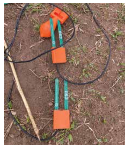
Soil moisture probes, useful for measuring the impact of drought on the Colorado River Basin, can be stationary or portable. Credit: Colorado Department of Agriculture
