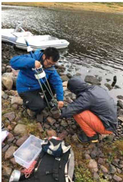
Boyang Zhao (left) and Tobias Schneider assemble a gravity corer at a lake in southern Greenland. Credit: Isla Castañeda
