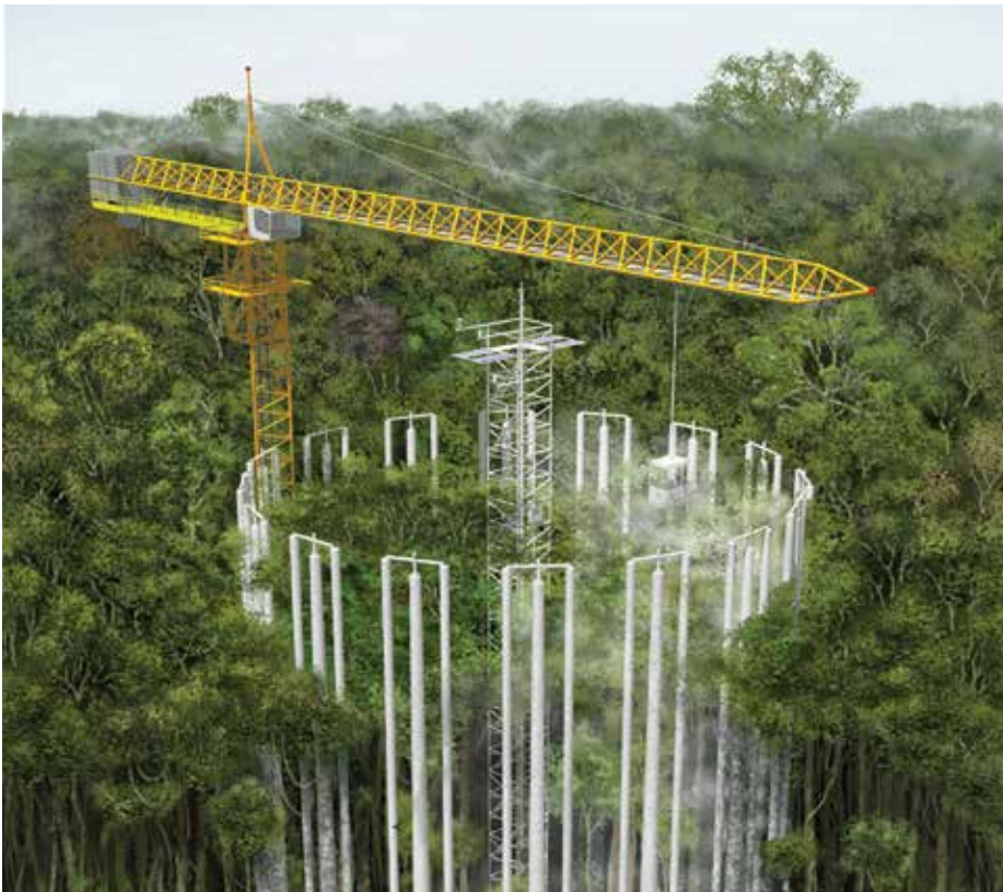
The AmazonFACE project, as shown in this artist's illustration, will involve a series of 35-meter-high metal towers injecting CO 2 into the tree canopy. Credit: P. Lorenzo & R. Lupo/AmazonFACE
