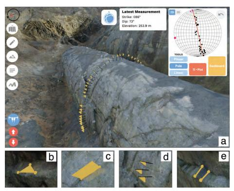
Users can place (a and d) orange flags, (b and c) planes, and (e) lineations on the virtual Whaleback to extract real-world data. Credit: Image adapted from Needle et al., 2022, https://doi.org/10.5194/gc-5-251-2022
