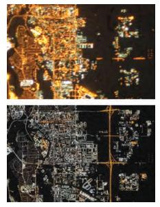
Astronaut photographs of East Calgary, Alta., Canada, show how city lighting changed from 2010 (top) to 2021 (bottom). Many streetlights switched from warm yellow-orange sodium lights to white LEDs, and new lighting was installed in residential areas and along highways. Credit: Earth Science and Remote Sensing Unit, NASA Johnson Space Center; georeferencing by GFZ Potsdam
