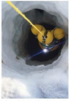
Icefin was pulled back up to the surface through a borehole drilled into Thwaites Glacier. Credit: Icefin/ ITGC/Schmidt
