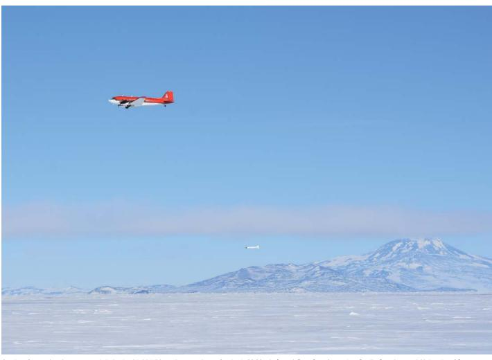
An aircraft tows the electromagnetic induction bird (visible at the center) over fast ice in McMurdo Sound, Ross Sea, Antarctica. Credit: Greg Leonard, University of Otago
