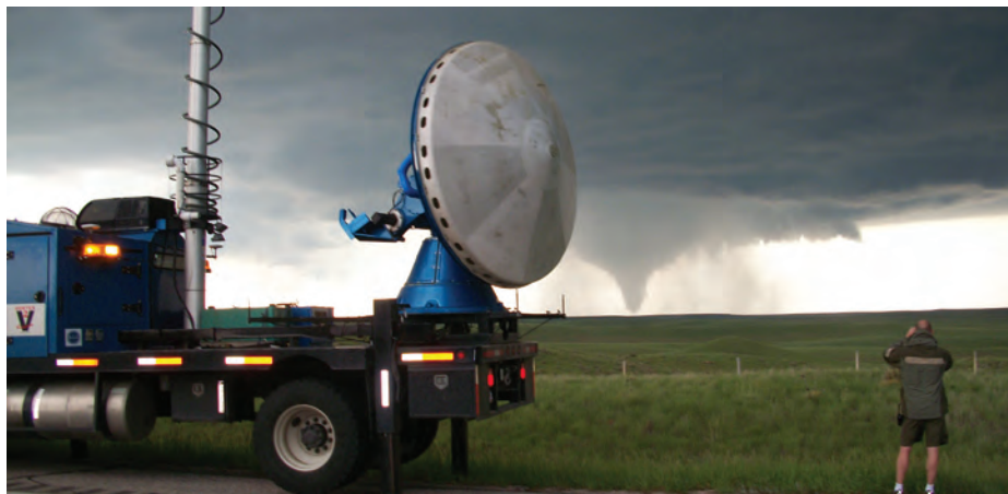
A set of radar instruments mounted on a truck, called a Doppler on Wheels, prepares to take measurements of an approaching tornado. Credit: Joshua Wurman
