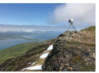
A new algorithm was shown to improve the use of data for earthquake sensing from Global Navigation Satellite System sensors, like this one on the Aleutian Peninsula of Alaska. Credit: Ellie Boyce/UNAVCO, CC BY 4.0 (bit.ly/ccby4-0)
