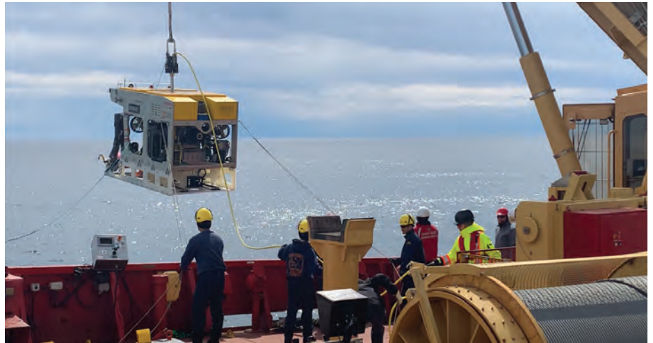
After refining seafloor maps, researchers searched for coral gardens with a remotely operated vehicle. Credit: Dave Cote, Fisheries and Oceans Canada
