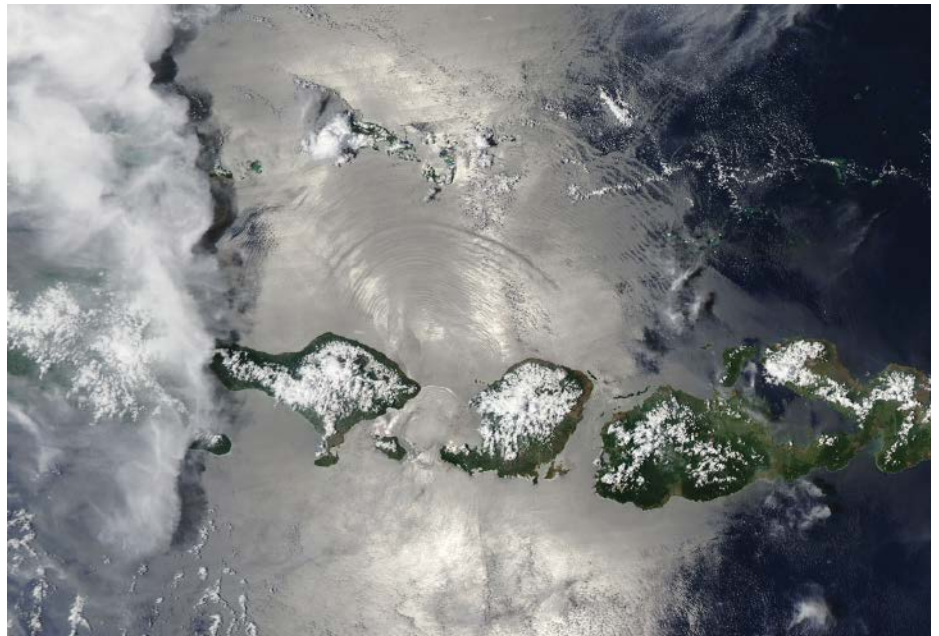
Internal ocean waves are generated when tides beneath the surface pass over seamounts, continental slopes, ridges, or other rough seafloor surfaces. The surface expression of such waves can be seen here in Indonesia's Lombok Strait because of the water's reflection of sunlight. Credit: Jeff Schmaltz, MODIS Land Rapid Response Team, NASA GSFC
