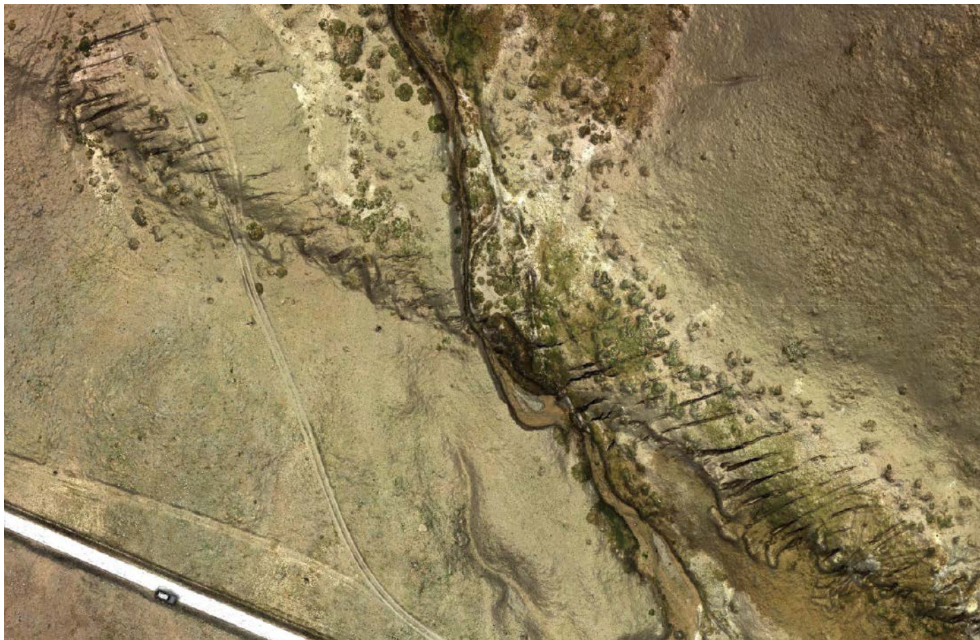
Researchers used unmanned aerial vehicle images superimposed on centimeter-resolution topography to study the surface rupture of the 2021 magnitude 7.4 Maduo earthquake in China. This image shows the fault scarp, tensional cracks on the hanging wall, and the left-laterally offset channel. Credit: Yanxiu Shao
