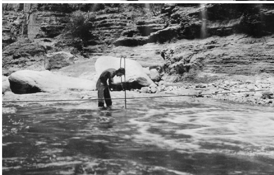
(top) U.S. Geological Survey hydrologist Eugene Clyde La Rue takes notes while in camp on Diamond Creek, a tributary of the Colorado River in Arizona, in 1923. (bottom) La Rue measures river discharge along Havasu Creek, another tributary in Arizona, also in 1923. Credit: Both: U.S. Geological Survey
