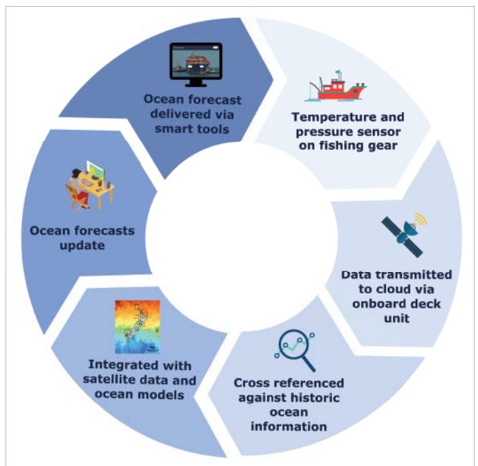
Fig. 2. The life cycle of ocean observations collected in partnership with the fishers. The observations are eventually fed into models that help provide forecasts of ocean conditions, which contain valuable information for fishers and other users.
