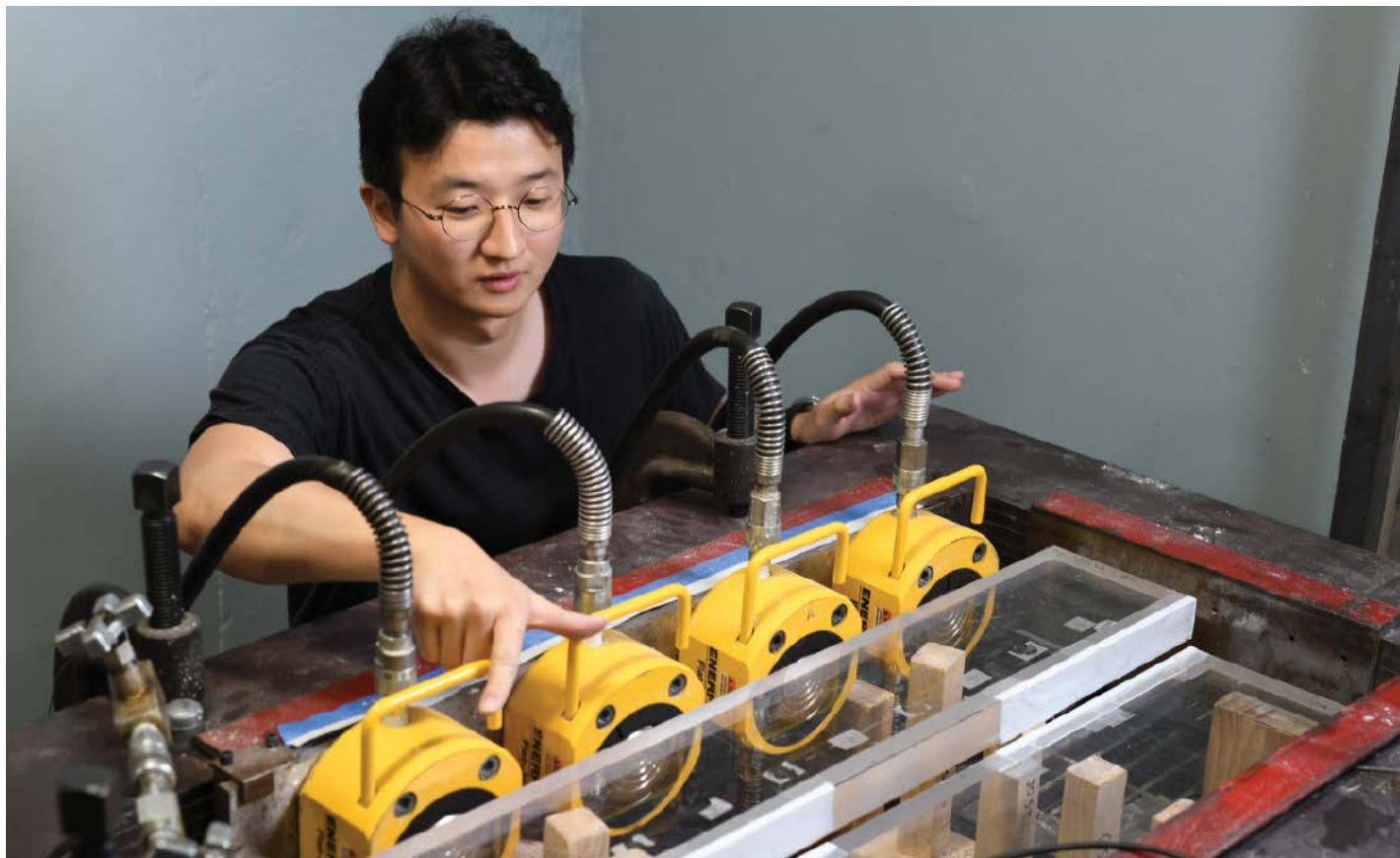
Scientists have discovered that coating some sections of plexiglass laboratory samples with Teflon can create confined ruptures that are similar to the way earthquakes occur on faults in nature. Here, Ph.D. student Jun Young Song prepares such an experiment. Credit: Gregory McLaskey
