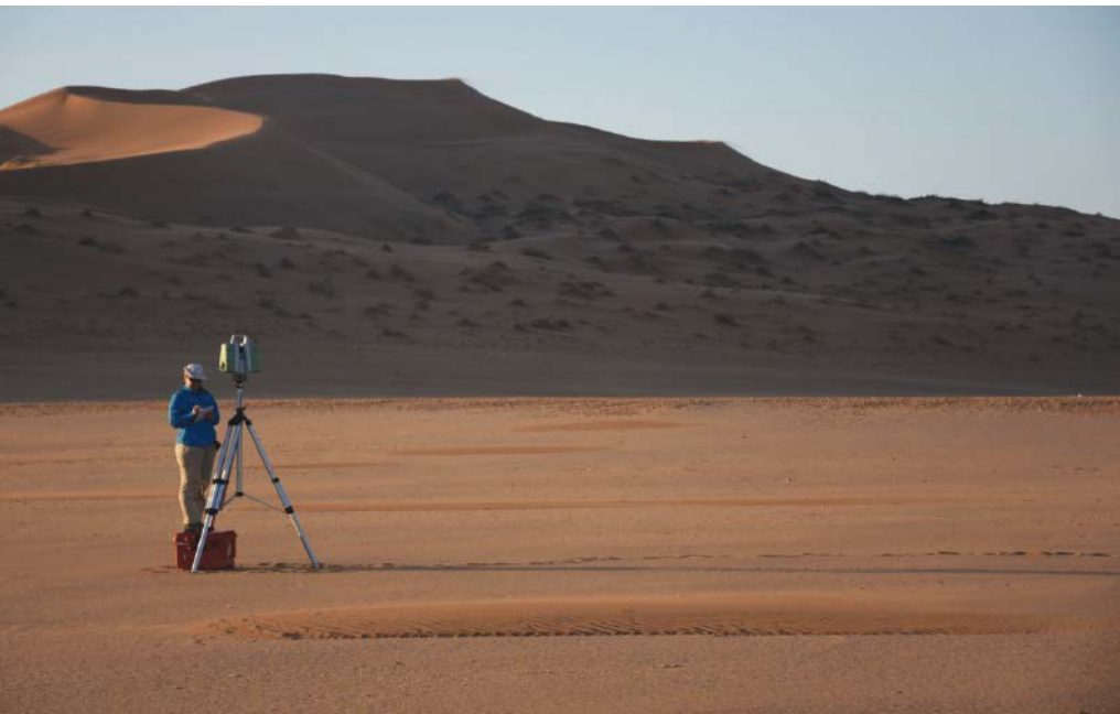
Geomorphologist Jo Nield uses a high-resolution laser scanner to study small dunes in Namibia’s Namib Desert. Credit: Matthew Baddock
