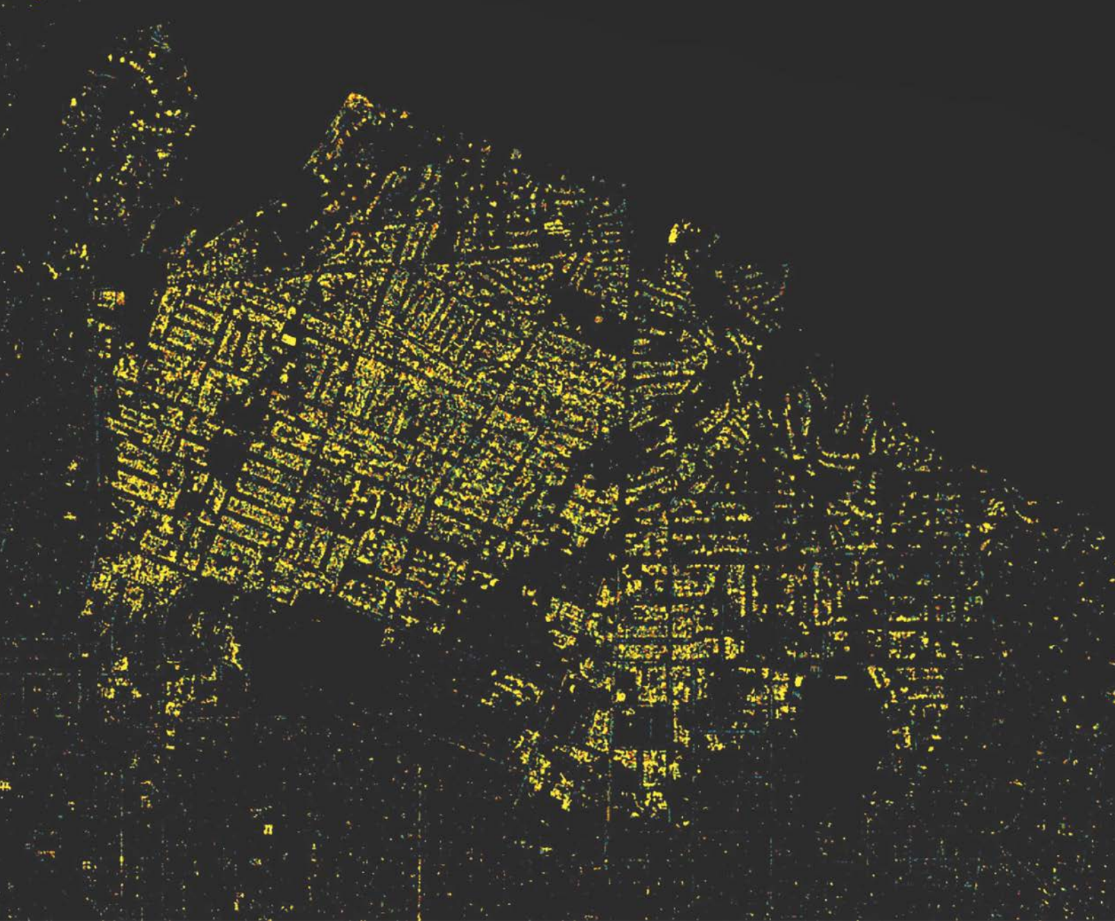
One of AVIRIS-3's quick-turnaround data products is this aerial map of the fraction of burn material, char, and ash within the spectrum of each pixel. Values from 0 (no burn, dark) to 1 (entirely burned, red) describe the burn fraction of the exposed surfaces. Nearly all structures have moderate to severe surface burning (yellow), and few pockets of vegetation (green) survive. Credit: AVIRIS-3/NASA/JPL, via Rob Green
