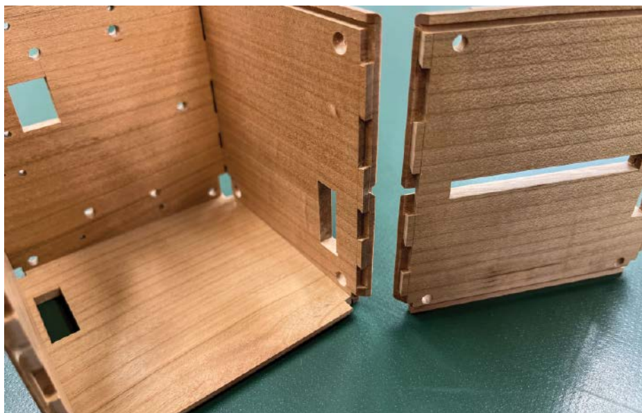
LignoSat was constructed using a traditional joinery method called the blind miter dovetail joint. Credit: Kyoto University
