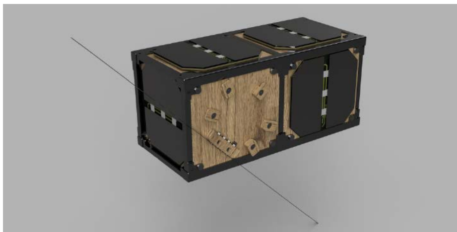
LignoSat-2 will have both an external and internal antenna and will be twice the size of the first LignoSat. Credit: Kyoto University
