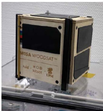
The WISA Woodsat contains a suite of sensors to measure how outer space will affect its materials. It also has a selfie stick. Credit: Arctic Astronautics/ Flickr, CC BY 2.0 (bit.ly/ccby2-0)
