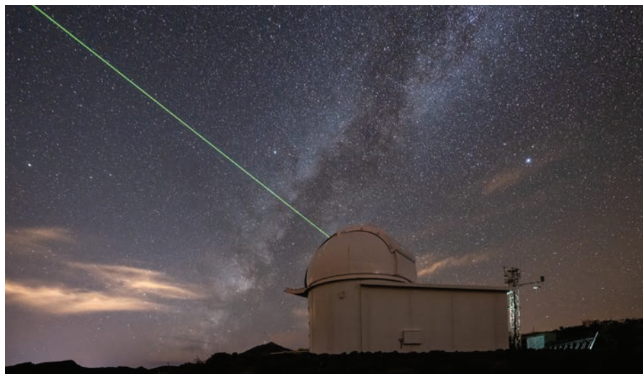
The European Space Agency’s (ESA) Izaña-1 laser ranging station at Teide Observatory in Tenerife, Spain, sends a green laser into space to detect, track, and observe active satellites. Credit: ESA
