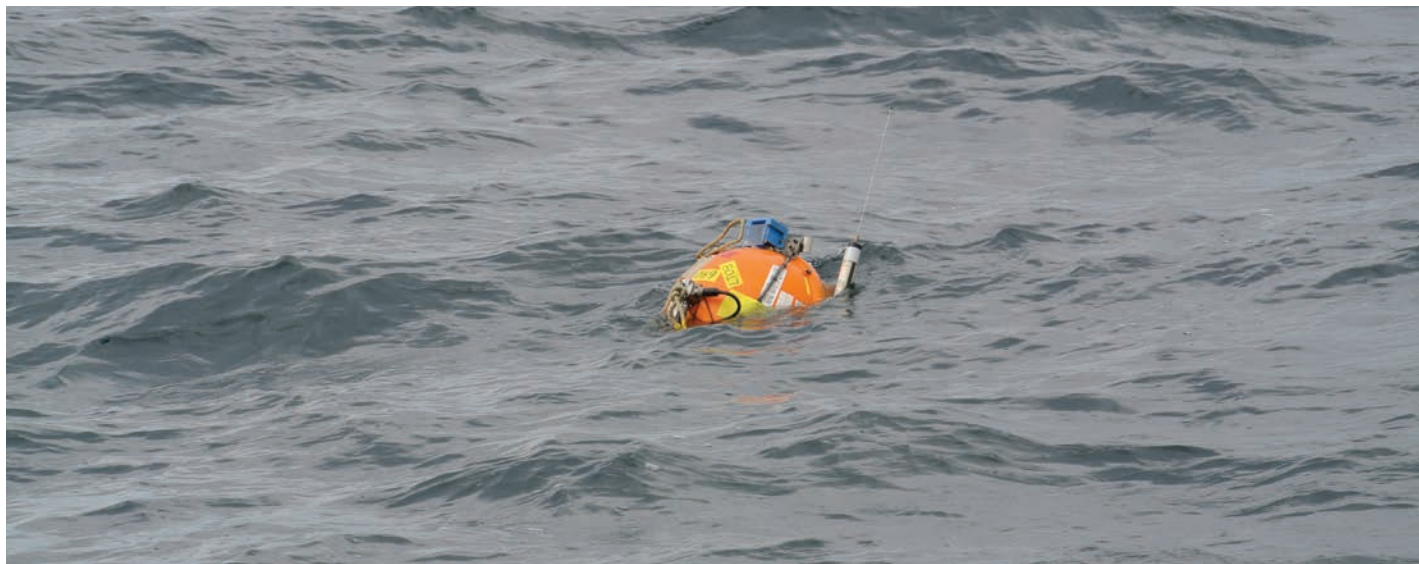
An ocean bottom seismometer emerges from the depths in 2021, after collecting 2 continuous years of data. The data were used to detect shallow tremors near the Chile Triple Junction, offering new insights into the development of the Patagonian slab window. Credit: Javier Ojeda
